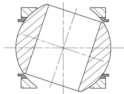
**The ring is made of special material and protects the seats against erosion.**
