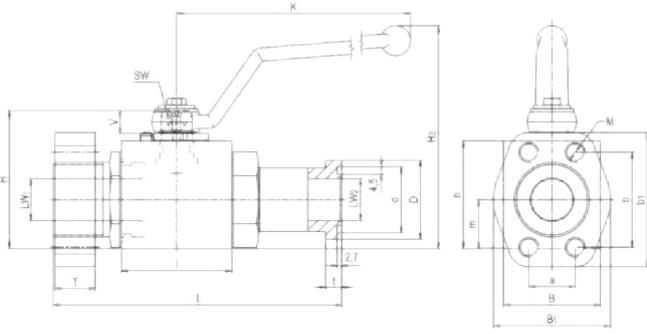
**High-Pressure Block Body Ball Valve - Type BBV-2-F/C3**
